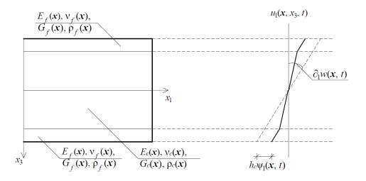
Figure 2 Assumed deflection along x1-axis direction
