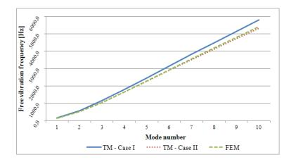
Figure 4 Comparison of free vibration frequencies obtained within all considered models
