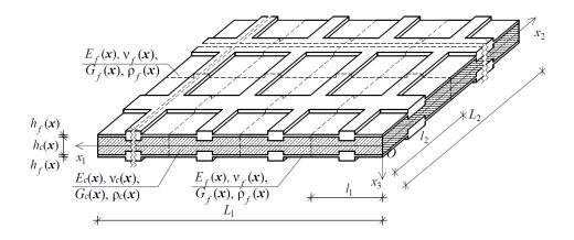
Figure 1 Sandwich three-layered plate with a certain periodic microstructure
