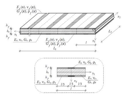
${\bf Figure}~{\bf 3}~{\rm A~sketch~of~considered~sandwich~plate~strip~with~a~details~of~a~basic~periodicity~cell$
